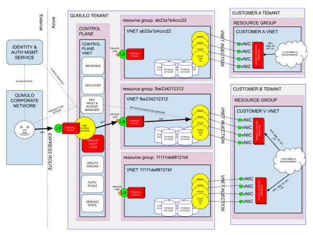
The control plane handles the automation of functions associated with a cloud service, including automated deployment and provisioning, monitoring and health checks, auto-scaling performance up and down, metering usage and submitting billing records to Azure. The service is designed to leverage cloud security best practices.
